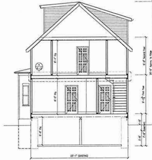
1 Living Room Building Cross Section SCALE: 1/4" = 1'-0"
